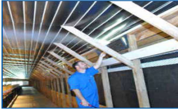
شكل (160) Using a smoke test to determine if air flow and operating pressure is correct
