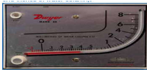
شكل (157) A manometer used to monitor air pressure within the house (the reading gieceeven is equivalent to 0.15 inches of water column)
